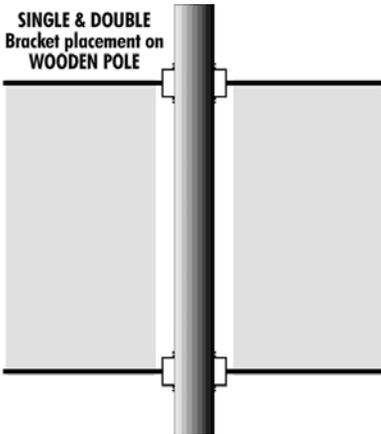
Position the point of the lag bolt inside the 12 o'clock bolt hole and drive it in with the impact wrench. Repeat for the 6 o'clock bolt hole.
